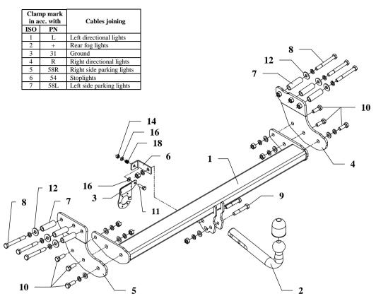
This towbar is designed to assembly in following cars: **VOLVO XC 90**, produced since 2003, catalogue no. **L18** and is prepared to tow trailers max total weight **2250 kg** and max vertical load **90 kg**.
